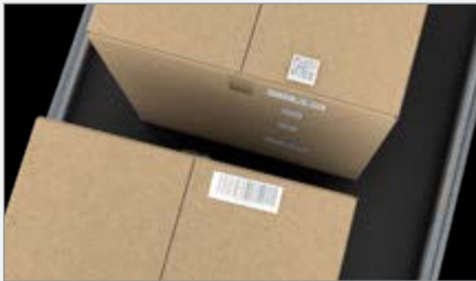
Short gaps between packages make uniform lighting difficult
