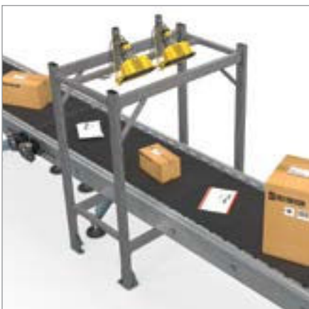
Single-sided scan tunnel
